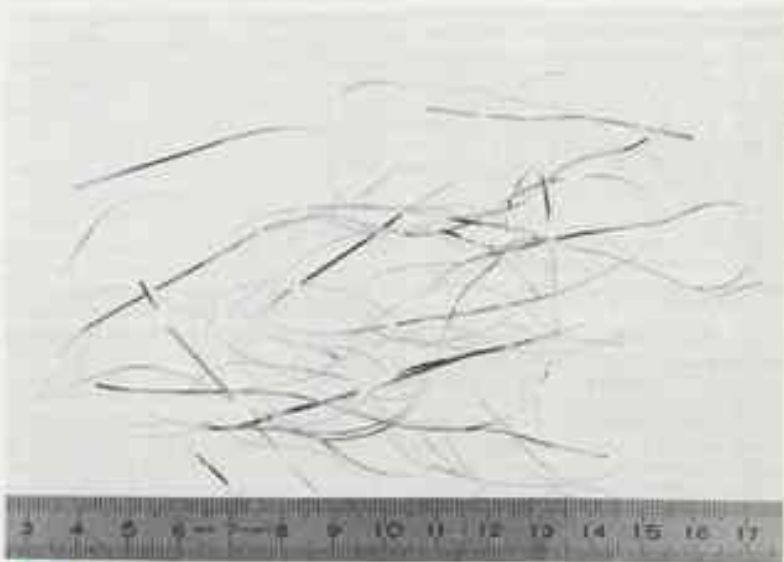
Figure 4 - Rubans Al-Cu-Ni-Mo amorphes.
