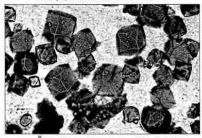
Fig. 2 - Synthise hydrothermale de spinelle NiAl<sub>2</sub>O<sub>4</sub> (700 °C, 2 kbar).
