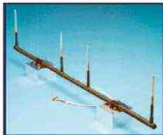
MIP electric antenna, 1m long, including two transmitting and two receiving electrodes (J. G. Trotignon)
