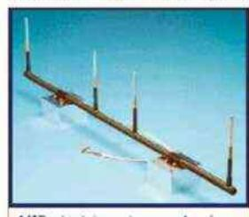
MIP electric antenna, 1m long, including two transmitting and two receiving electrodes (J. G. Trotignon)
